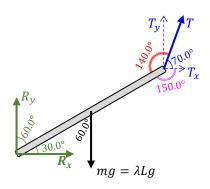
7b) For reaction forces, I want to split up all forces (including tension) on a standard xy-coordinate system. We do it this way since almost everyone splits the pivot reaction force into  $R_x \& R_y$  with standard xy-coordinates. Do *horizontal* sum of forces:
