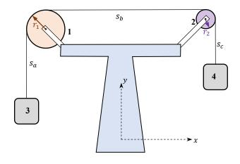
4c) If the string is inextensible, and both masses are connected to it, both masses accelerate with same magnitude. The accelerations can be different if using different strings attached at different radii (or if the string is extensible).
