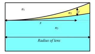
4) A cross-sectional view (right half only) of an unusual camera lens is shown. The lens is designed such that the surface between materials 1 and 2 is described by the equation  $y=ax^2$  where y is the height above the horizontal axis shown. The surface between materials 2 and 3 is the top of a plano-concave lens with radius of curvature 2.00 m. The radius of the lens is 30.0 cm.
