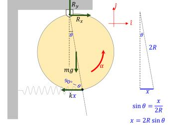
Using a right hand rule, one sees the torques exerted on the sphere by mg & kx are in the  $-\hat{k}$  direction. Sum of torques gives:
