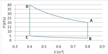
\*\*\*\*\*\*3a) A PV diagram is shown for a Stirling engine. The engine uses a diatomic gas between 100K and 1000K.
