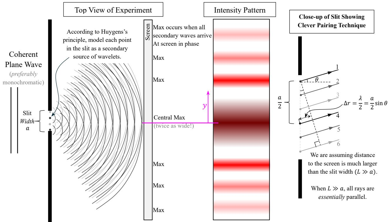
Consider the *rightmost* figure above showing six secondary wavelets produced according to Huygens's principle.
