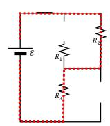
8b) When the circuit reaches steady state, the two inductors acts like shorts. In steady state, we see resistors  $R_1 \& R_2$  are in parallel while resistor  $R_3$  is bypassed by the inductor (which is acting like a short).
