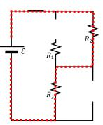
8b) When the circuit reaches steady state, the two inductors acts like shorts. In steady state, we see resistors  $R_1 \& R_2$  are in parallel while resistor  $R_3$  is bypassed by the inductor (which is acting like a short).
