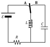
An *LCR* series circuit is built using a 3.00 mH inductor, a variable capacitor set to 222 nF, and a 470  $\Omega$  resistor. The function generator used to drive the circuit produces a sine wave with voltage amplitude 12.00 V. Phase angle when using these parameters is  $-56.7^{\circ}$ . For the following, circle the best answer or answers (all which apply). 8a) Which circuit element is dominating this circuit?
