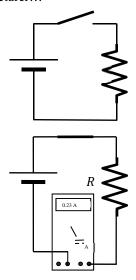
Measure the following quantities with an OPEN SWITCH (open circuit):
